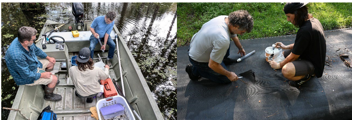
Plate 3a. (left) Boat-based sediment sampling in Squash Branch, October 2024. Plate 3b (right) Sampling of geotubes on shore for phosphorus.
